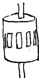
The “Lantern”, with openings to take the teeth of the big wheel.
